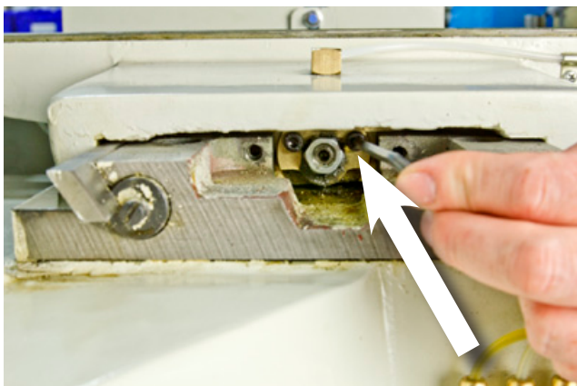
Set Screw Adjustment on the Y-Axis
