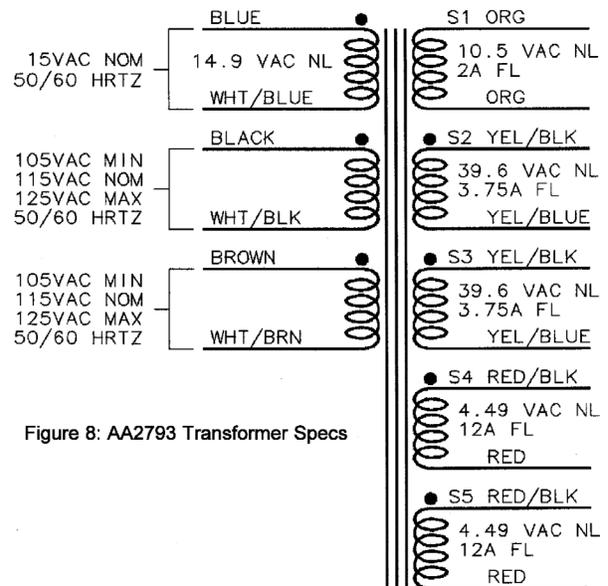
Figure 8: AA2793 Transformer Specs
