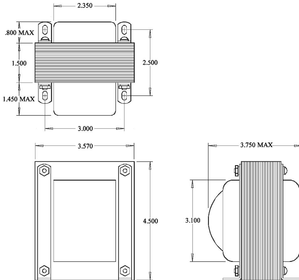
Figure 6: Transformer Dimensions
