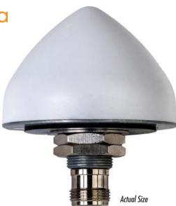
The Model 8230 is a high gain (40 dB) GNSS outdoor antenna covering GPS L1, GLONASS L1, BeiDou B1, Galileo E1, and QZSS L1. It uses a three stage low noise amplifier, a mid-section SAW, and a tight pre-filter to protect against saturation by high level sub-harmonics and L-band signals.
