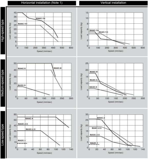
(Note) In the above graphs, the number after the type code indicates the lead. (Note 1) The figures for horizontal installation assume use of an external guide.
