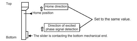
(Example 2) The power is turned on when the slider is contacting the bottom mechanical end in a configuration where the motor is positioned at the bottom.
