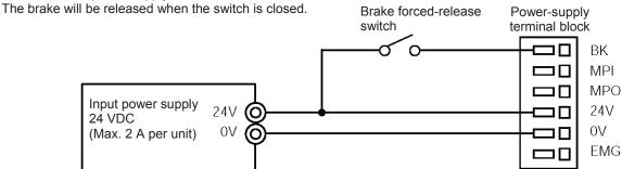
Danger: If the actuator is oriented vertically, exercise due caution when releasing the brake to prevent the slider/rod from dropping unexpectedly to pinch your hand or damage the robot hand or work.
