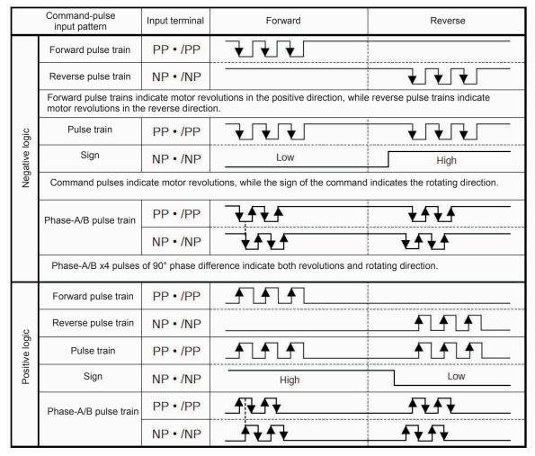
(Note) The figures shown above are an image when a command pulse input is made on the differential line driver.
