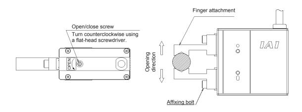
[Three-finger type] Remove one of the finger attachments.
