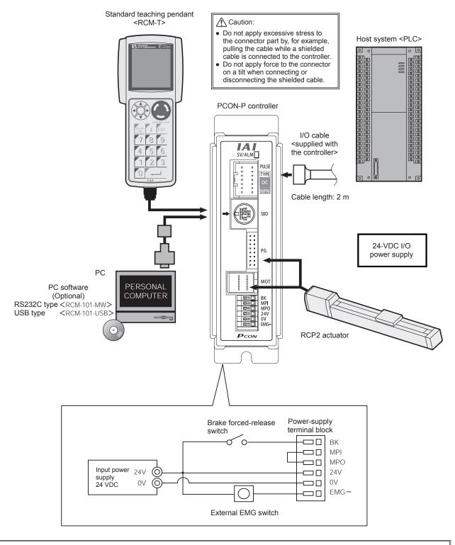
⚠ Caution: The BK terminal need not be connected if the actuator has no brake.
