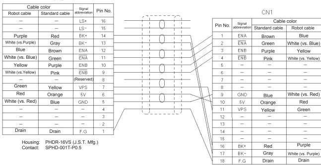
Housing: XMP-18V (J.S.T. Mfg.) Contact: BXA-001T-P0.6 Retainer: XMS-09V
