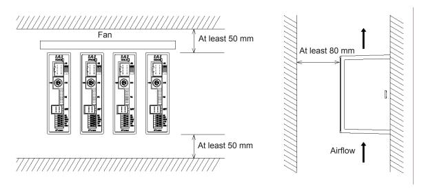
Regardless of whether you are installing one or more controllers, provide sufficient clearances around each controller to permit easy access for installation and removal of the controller.
