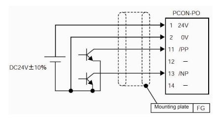
Note 1 Always connect the shield of the twisted pair cable joined to the connector, to the mounting plate.
