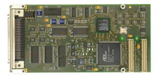
The 8 analog output channels are realized by eight 16 bit digital to analog converters (DACs). The conversion time is 10 µs. An operational amplifier drives the full-scale range of ±10V and is capable to drive high capacitive loads. Similar to the analog inputs a sequencer can control the analog outputs.
