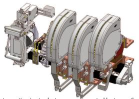
Contactor with single interruption in air, electromagnetic control by two coils (one for close and one for open), and also handle lever.
