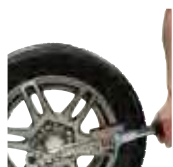
Completion of tightening process with Blue signal.
