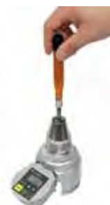
BMRD torque checking with BTGE-G.
