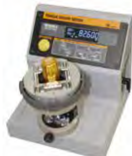
Click type RTD with TDT3-G and loading device STA.
