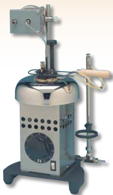
Pensky-Martens flash point tester 59871-00 shown with motor 59871-50
