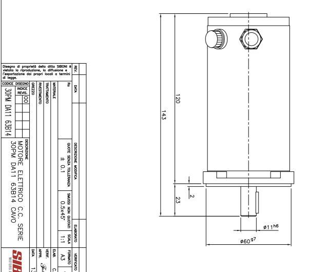
MOTORE ELETTRICO C.C. SERIE 30PM DA11 63B14 CAVO
