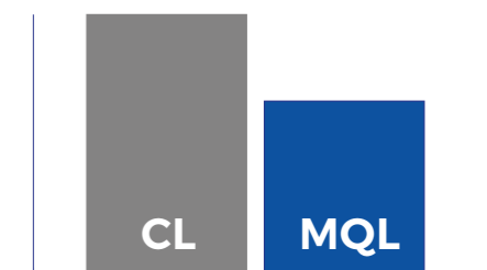
With HPM Breeze, the spindle load is decreased by approx. 30%
