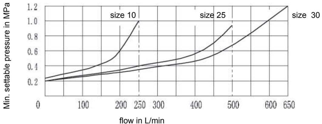
The characteristic curves are valid for outlet pressure  $B = 0$  over the entire flow range!
