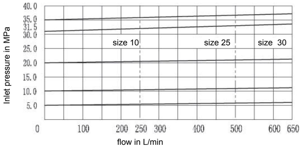
Minimum settable pressure and bypass pressure in relation to the flow
