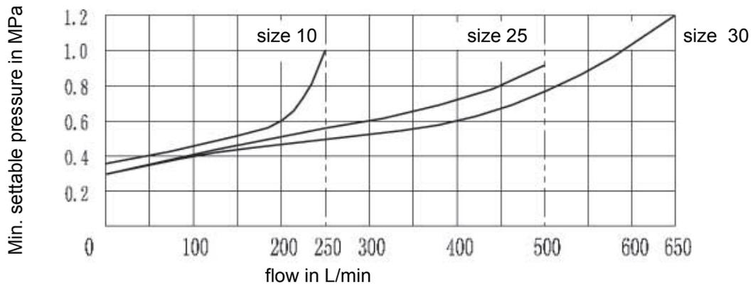
Minimum settable pressure and bypass pressure in relation to the flow
