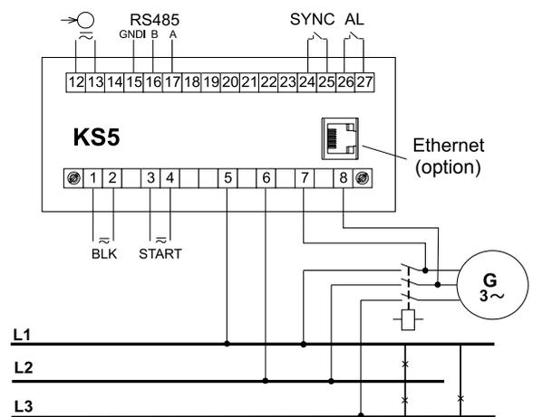
Meter connections - measurement phase voltages
